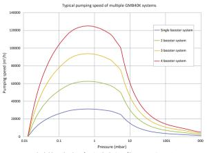
Scalable technology for simple design of large pumping systems or adding redundancy to valuable processes.
